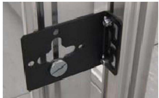
L-Shaped Bracket on Upright Frame Member
