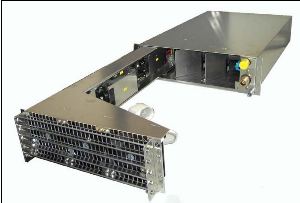
figure fan unit completely pulled out
